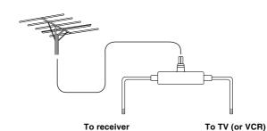
Connecting the antenna cable to the 75/300  $\Omega$  antenna adapter (For all models other than USA, Canadian and European models)
